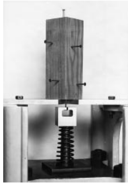
FIG. 36 Nail Withdrawal Test Assembly Showing Specimen in Position for Withdrawal of Nail Driven in One End of the Specimen
