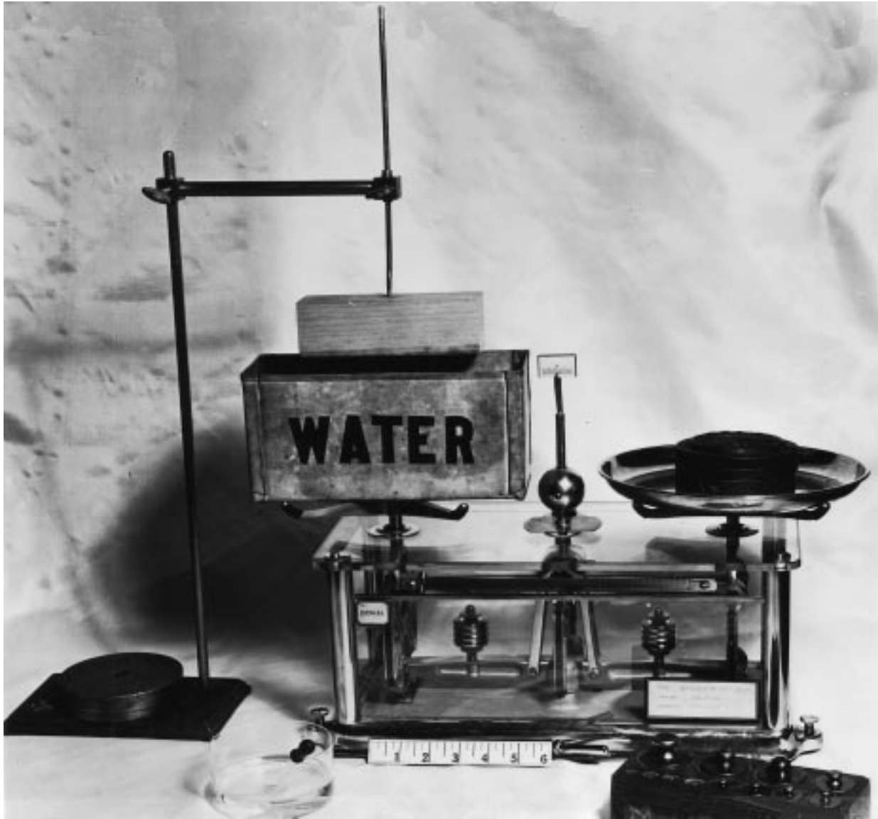
FIG. 39 Specific Gravity and Shrinkage-in-Volume Test Set-Up
