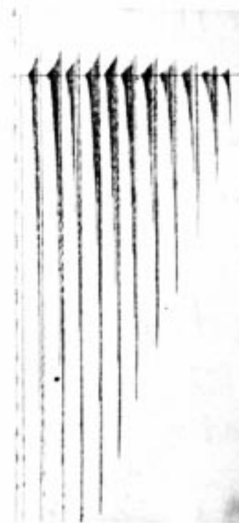
FIG. 12 Sample Drum Record of Impact Bending Test
