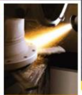
Twin wire Electric Arc Spraying
