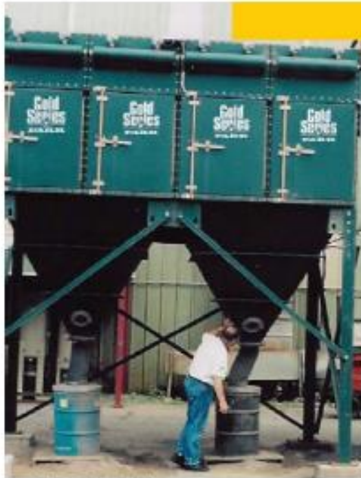
GS 48 on RR Car Sand Blasting
