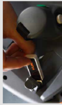
A USB port integrated into the housing allows the saving and loading of configurations directly on the smartPAD.
