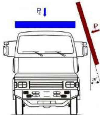
Figure 3 Roof strength test (Test C)
