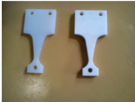
Figura 9-2 Probetas
