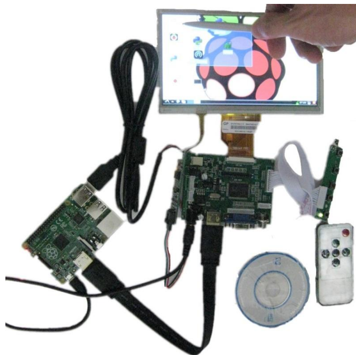
Figura 4.17 Interface entre Raspberry Pi con LCD touch 7". Fuente: http://www.aliexpress.com/item-img/7-Inch-TFT-Touch-Screen-LCD-Monitor-For-Raspberry-Pi-Driver-Board-HDMI-VGA-2AV-Provide/1846532213.html .
