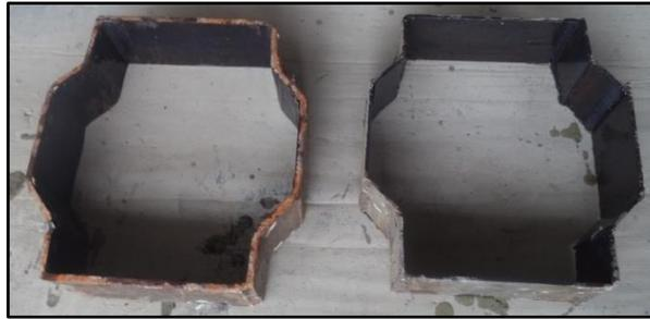
**Fig. 32:** Moldes adoquines
